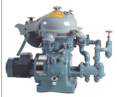
Fig 1. MAB 104B-14/24, with feed and discharge pump.
